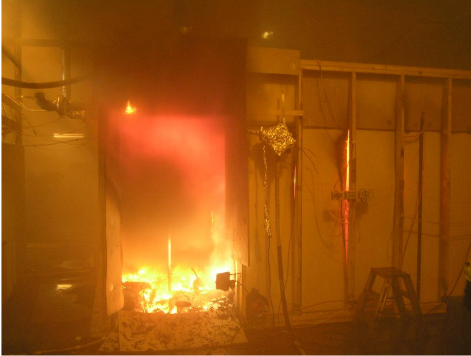
Figure 10. Flashover fire test, where the flames are spread in the corridor from the burning cabin.
